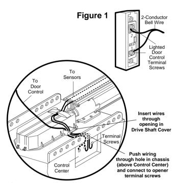
Figure 2 WIRING TO CONTROL CENTER
